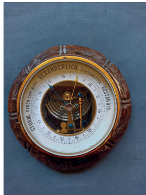
Abb. 3: Barometer HF, Facettenglas, Papierskala, 1895.
